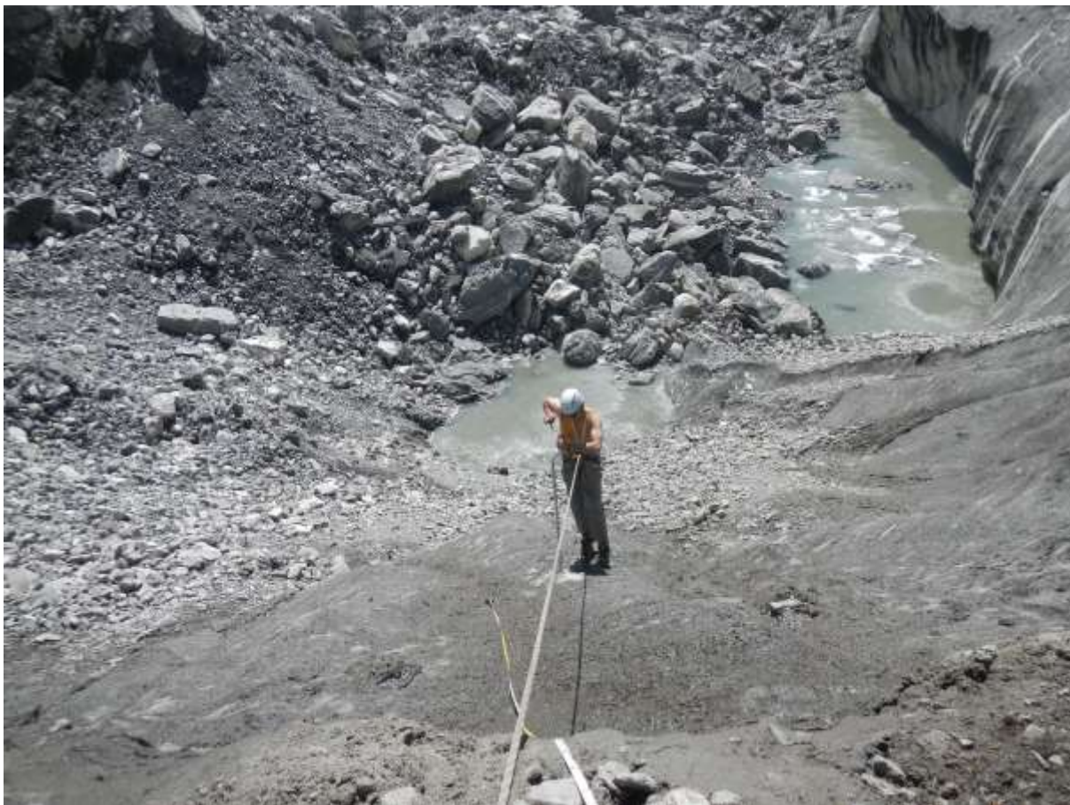
Me, drilling into an ice cliff adjacent to a small lake to determine the rate of the lakes expansion.
